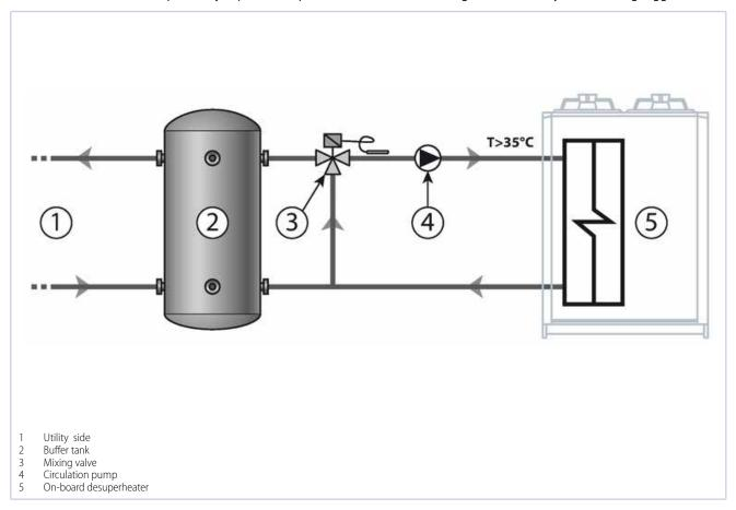
The bulb of the 3-way mixer valve is placed at the de-superheater exchanger inlet. By mixing the hot water produced by the recovery with colder water from the tank, it reduces the time needed for the system to reach full operating capacity to a few moments. A buffer tank must be placed between the unit and the utility since the demand for hot water and its availability are not simultaneous, because it needs the compressors to be running.
